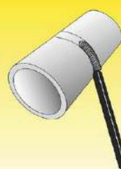
Pipe fixed with axis horizontal, welding downwards: PG/5G
