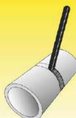
Pipe fixed with axis horizontal, welding upwards: PH/5G
