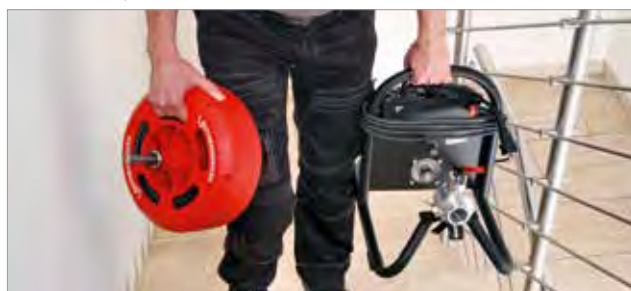
Convenient transport thanks to detachable drum
