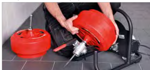
Interchangeable drum for different working ranges
