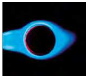
High flame temperature based on cyclone swirl
