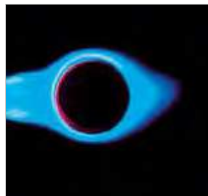
High flame temperature based on cyclone swirl
