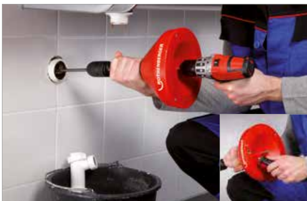
Electrical operation with cordless drill
