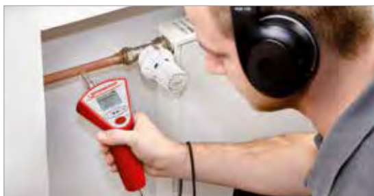
Acoustic leak detection of heating installations
